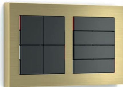
E12 - 4-fold pushbutton and room thermostat - Deep double plate. 4 square and 4 rectangular horizontal rockers. Rockers: finishing brushed metal, carbon colour. Plate: finishing brushed metal, brass colour, red/white LED. Dimensions: mm 87 x 158 x 9
